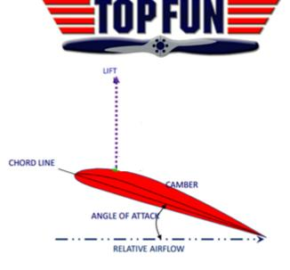
With any generation of lift also means creation of drag.
